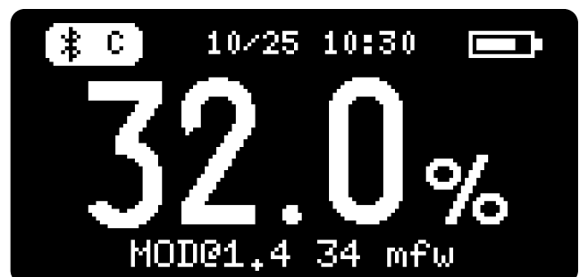
Fresh water, metres: 34 mfw.
