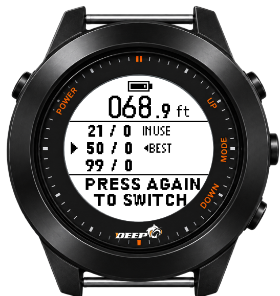
Gas switch - confirm
